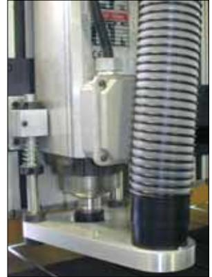
The pressure foot is ideal for plastics, woods, composites, fiberglass, or any substrate when routed. The pressure foot fits any manual high-frequency collet type spindles. This accessory can be added at any time.
