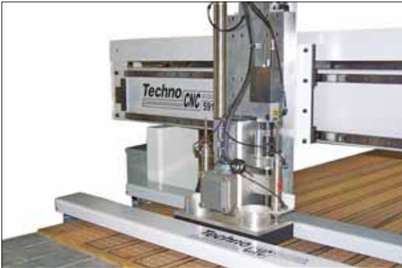
Techno's roller hold-down system is designed to work on Techno Premium Class CNC router models. It is ideal for rough plywood or stacked sheet materials when the conventional vacuum hold-down is not practical enough to do the job. Now two and three sheets of material can be processed allowing an even shorter manufacturing cycle time. The twin roller positions applies maximum downward force to the material, preventing part slippage.
