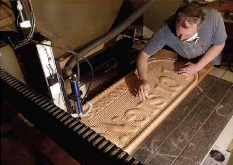
*The Techno router makes it possible to produce 2D and 3D images faster and with more accuracy.*
