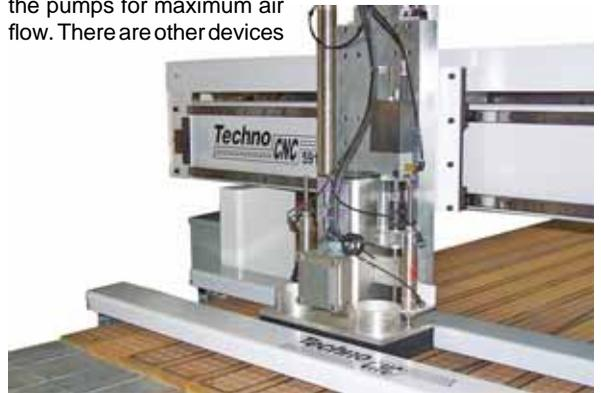
which can be purchased to aid the vacuum hold-down system such as a spindle pressure foot, or roller hold-down. These devices push down on the material while being routed thus aiding the vacuum system.
