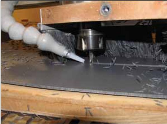
The main drawback of using a cold air gun is that a fairly large compressor is required. This need for a substantial compressor does add to the overall cost of the unit.
