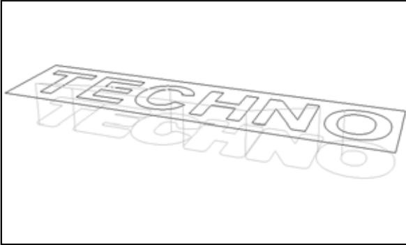
For instance, a 2D part only requires that the depth of the cut be specified along with the path once the tool reaches the desired depth. When a 3D part is being carved, the full program description can consist of hundreds of thousands of G-Code commands specifying the toolpath. The program for 3D parts usually consists of very small line segments that form the desired shape.
