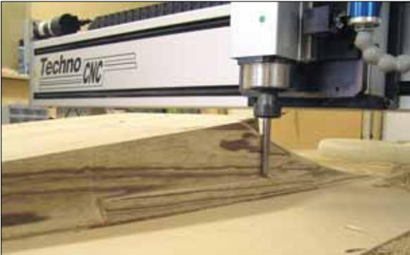
CNC automation enables you to design a part on your PC, and then reproduce that design quickly and easily using the router. There are three basic steps to this process. First, a computer image is generated, typically through a CAD program. Second, a CAM program translates the geometry of the CAD drawing and cutter compensations to output a toolpath. And lastly, the toolpath is converted to a manufacturing programming language (i.e., G-Code) used
