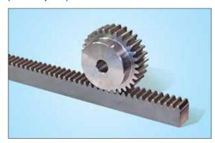
Some CNC Routers use other drive systems, such as the rack-and-pinion gear drive. The racks are typically installed on the outside of the machine, thus exposed to the elements. As the machine cuts, debris collects on the rack. These foreign materials get ground into the racks and gears, causing more friction in the drive system which, in turn, causes wear and makes the machine less accurate and unstable.
