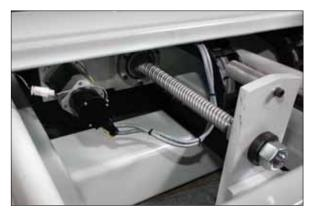
Servomotor resolution depends upon the encoder used. Typical encoders produce positional signals (or pulses) per revolution, and encoders range from 500 to 200,000 pulses per revolution. The more pulses there are, the finer the resolution capability of the motor. Servos can perform highspeed continuous motion much more reliably because of the constant feedback from the encoder, making them much better suited to applications requiring a high-end quality finish.
