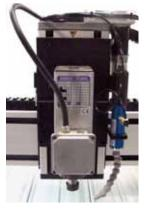
zero the Z-axis. Although this is not difficult, the task had to be performed carefully or else the second tool would not be at the correct height and the part might have a visible defect. Now, all Techno machines and many other CNC machines come with tool-length sensors and compensation software. This allows for the tool length to not only be measured but automatically compensated for in the G-Code software, with a simple and automatic process.
