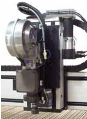
Compressed-air-cooled spindles allow for a 90% duty cycle. These require a constant stream of clean nonfluctuating source of compressed air. These spindles are typically used for greater than 24,000 rpm. These spindles usually incorporate ceramic bearings.
