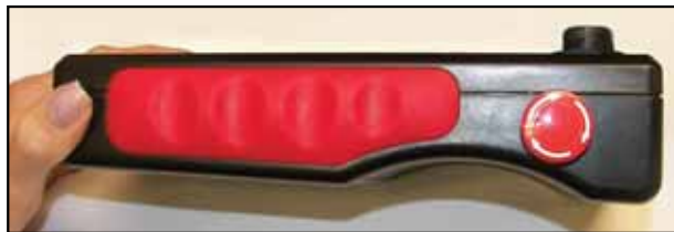
Top View A.R.T. Controller showing external Emergency Stop Button
